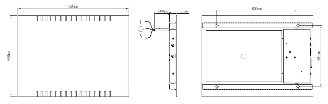
Remarks: The fixing sizes are same as the horizontal mirror (10015), but one is horizontal installation, another is vertical installation
